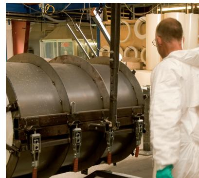
The result of this process is a viscous foamy casting material which quickly transforms into solid form PUR. The PUR can be generated with a variety of rigidity and density. When the liquids are injected into special moulds, it is possible to cast insulation shells and block foam.
