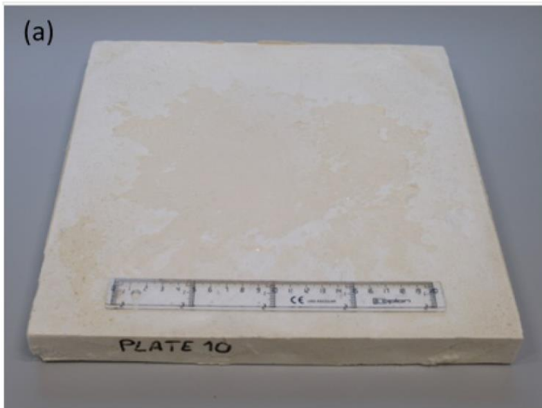
(a) Plates of rigid polyurethane foams with 3 wt% and (b) 10 wt% of recycled polyurethane foam powder.
