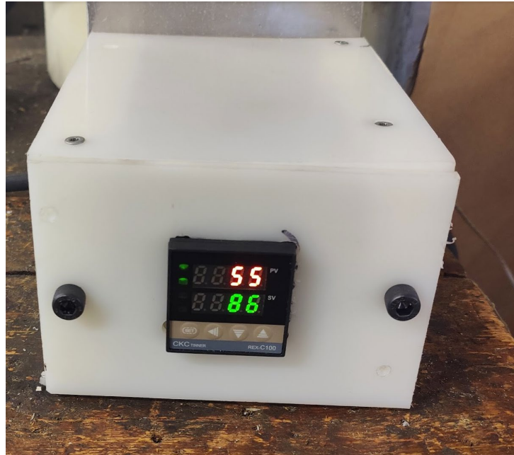
Figure 7: Photo of the PID controller used for the test showing actual (upper) and target (lower) temperature values.
